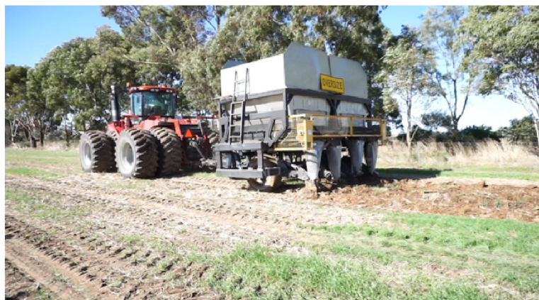
Figure 4. Terra Nova's 4m Subsoiling Machine first run with amendment.
